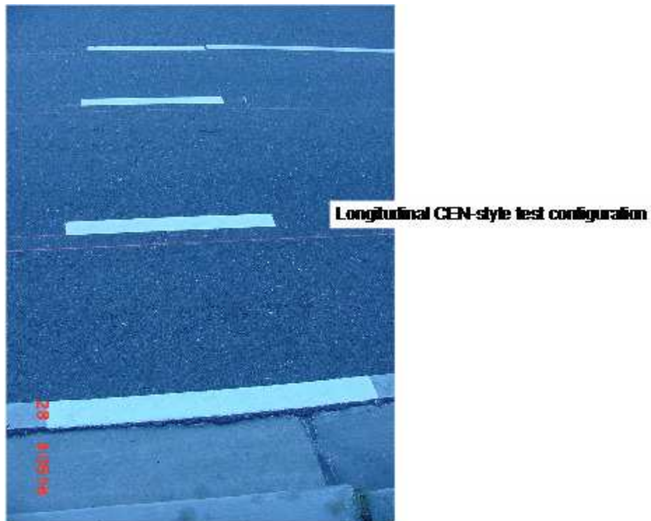
Figure 2. CEN-style test deck configuration on the New Orleans Highways for Life Test Deck.
