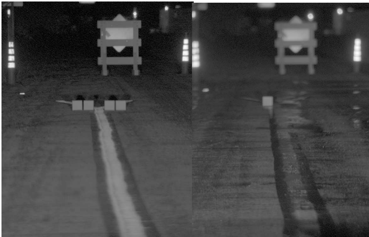
Figure 31. Screen captures from imaging photometer showing Reference 1 at a distance of 45m under dry (left) and rain (right) conditions.
