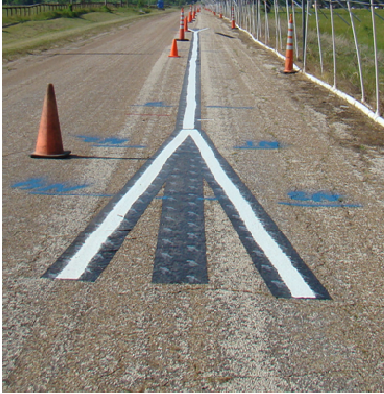
Figure 8. Experimental pavement marking applied to black polymer film to allow easy removal of the test markings after completion of the Task 2 experiment
