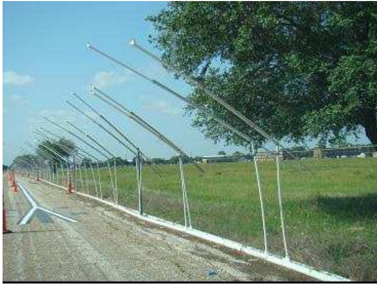
Figure 16. Close up view of sprinkler system used to produce artificial rain on the TTI Rain Tunnel, viewed from north end of Bryan Road.
