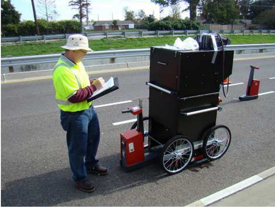
Figure 6. EN 1436 rain simulator
