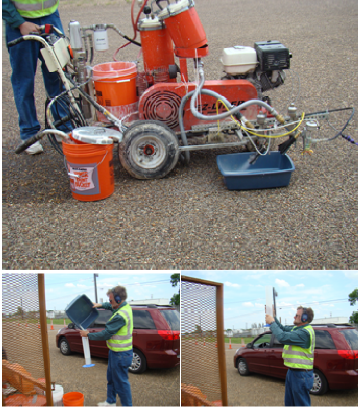
Figure 10. Calibration of Element and Glass bead application rates
