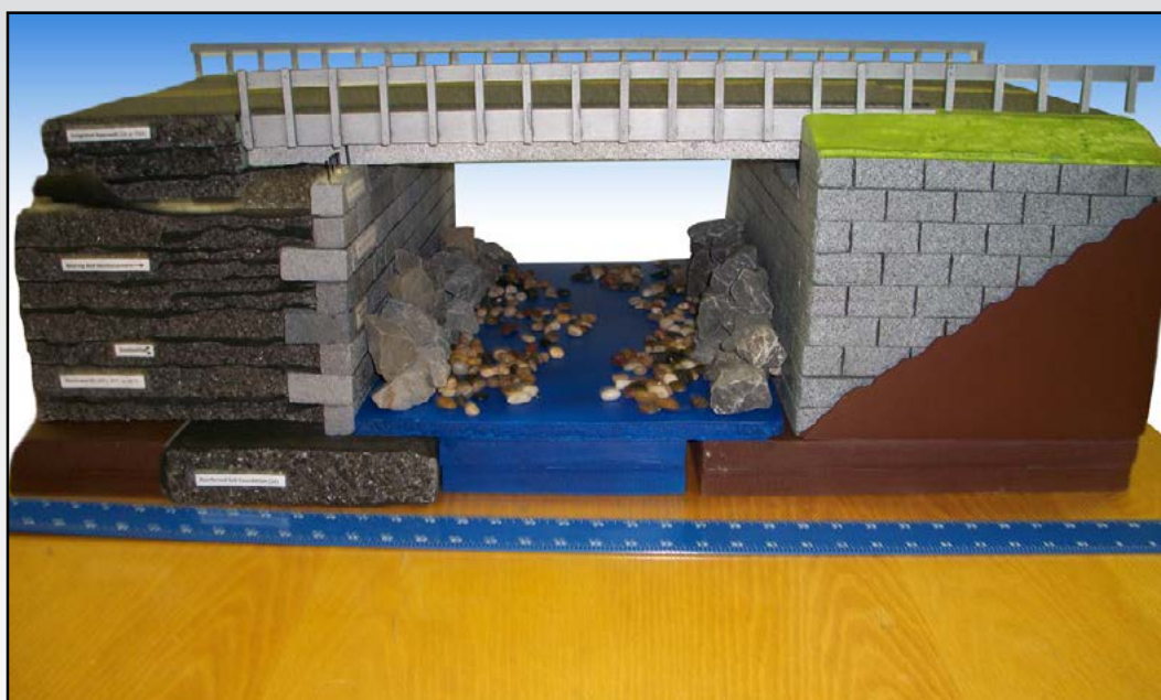
The Pennsylvania DOT is using a traveling tabletop model to demonstrate the benefits of geosynthetic reinforced soils in bridge construction.
